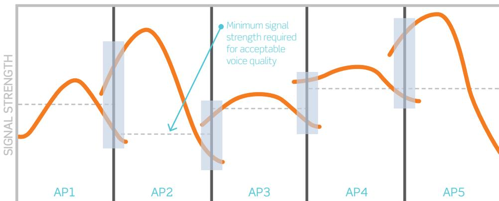
**Figure 2: Voice over Wi-Fi hand-off optimized for the enterprise**
