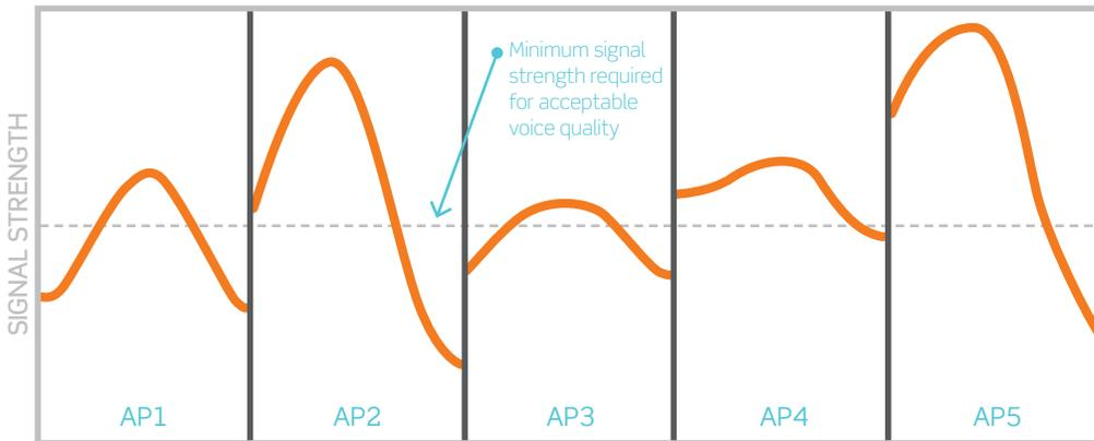
**Figure 1: Typical smartphone AP hand-off in the enterprise**
