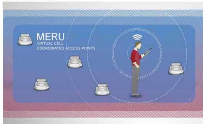
Virtual Cell – Provides 'zero-handoff' seamless roaming.
